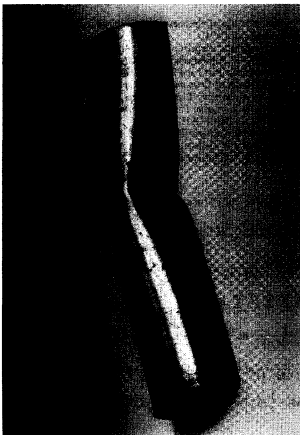
Fig. 13. Local elastic-plastic dent of pipe P_7 .
